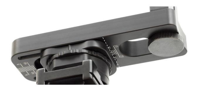
**example (continued):** Based on the mm scale on the underside of the lower rail, the previously determined value of approx. 21.5 mm is set. To do this, match the edge of the sliding part (either left or right, depending on the value) with the desired value on the mm scale.
