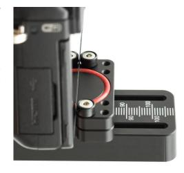
**Version with Arca-Swiss clamp (VARIO-K):** When mounting the camera, make sure that the clamping plate is exactly in the center of the clamp (the clamping plate used should have a center mark). After tightening the clamp, check that the camera is securely and firmly clamped before releasing it.
